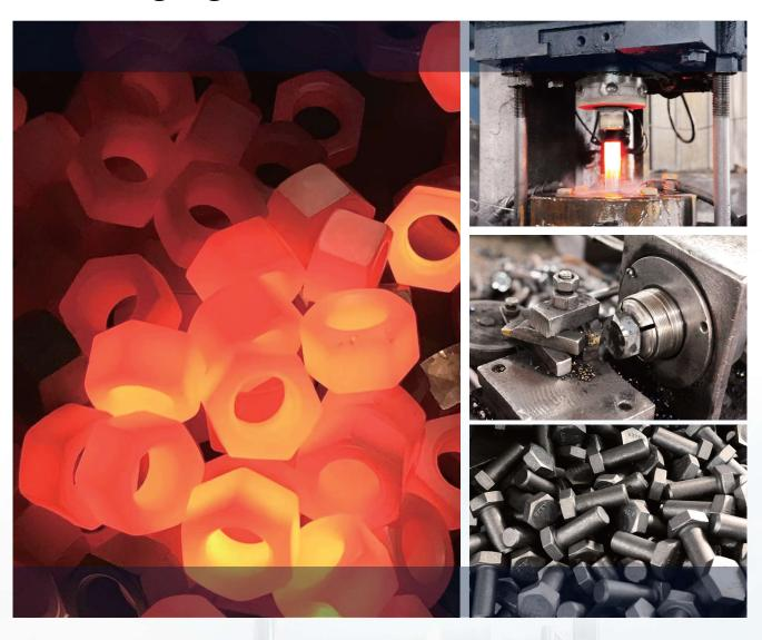
Raw Material - Bar Cutting - Hot Forging - Chamfering Machine-Sand Blasting - Thread Rolling/Tapping - Heat Treatment - Coating - Packing 一亿多金属———
