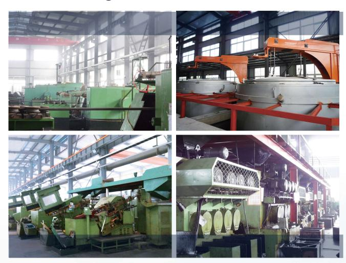
Raw Material - Spherroidizing Annealing - Acid-Picckling - Wire Drawing - Cold Forming - Thread Rolling/Tapping - Heat Treatment - Coating - Packing
